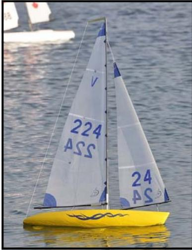
The Victoria Class is one of the largest, least expensive and most popular R/C model yacht classes in Canada. Fabricated of ABS plastic, it is simple to assemble and easily transportable in the family car to sailing venues.
